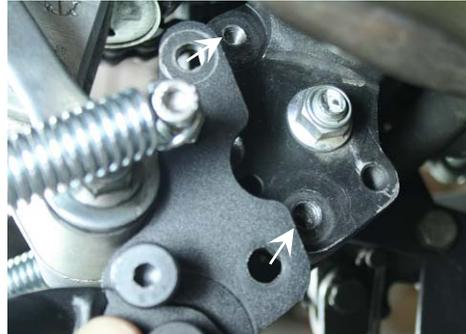
Place the 10mm washer onto the 10mm bolt, and the 8mm washer onto the 8mm bolt. Set the bolts, washers and spacers nearby as they will be necessary soon. Use one hand lift the center stand into position, aligning the mounting holes on the center stand with the mounting holes on the frame. Unlike the previous step, insert the 10mm bolt and washer BOTTOM mounting hole on the center stand first. Slide one 13/32" long x 3/4" OD spacer behind the bolt and thread it into the hole by hand.
